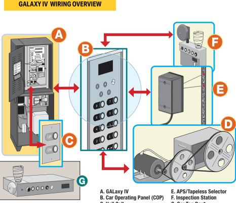
\*NOTE: Controller can be configured for traveling cable connections to Car Top Box or Car Operating Panel
