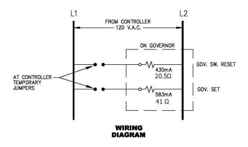
Setting the governor is accomplished by activating a solenoid at any speed less than normal overspeed, thus setting the grips and activating the safety.
