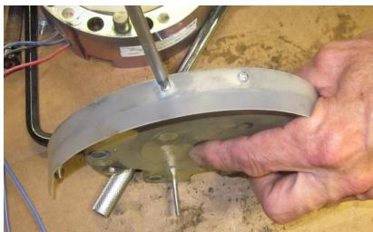
• Remove Compression Springs (8), Compression Washers (8), Brake Lever Spring, and Plastic Brake Shield.
