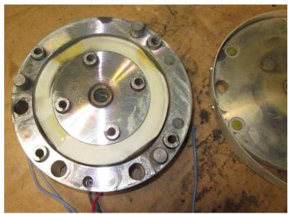
• Release C-Clamps evenly and remove Brake Shoe Plate from Coil Assembly
