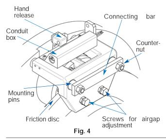
Mount the mounting pins, then the connecting bar and tighten with the indicated torque for the locknuts
