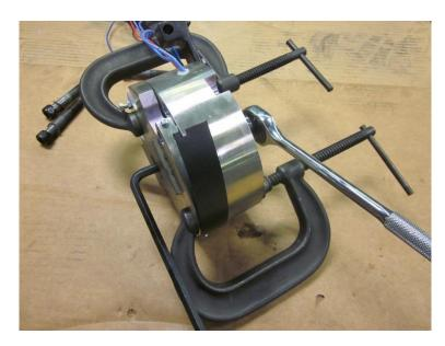
• Clamp Brake Coil Assembly shut with 2 C-Clamps.
