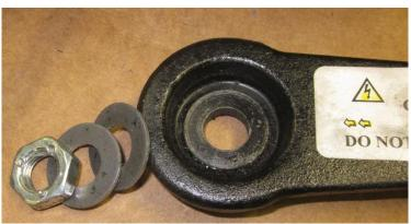
• Unbolt the Brake Release Lever. Note; this bolt is under some spring pressure. Care should be taken when releasing. Take note of small parts and ball bearings.
