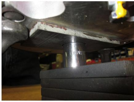
• To reassemble the Brake Lever, use the 18mm Socket to help compress the Brake Lever Bolt to get the nut started.
