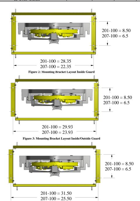
Figure 4: Mounting Bracket Layout Outside Guard
