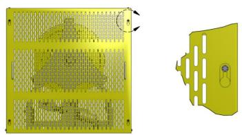
Figure 6: Access Panel Attachment
