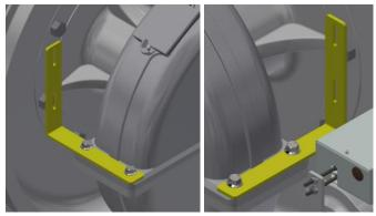
• Attach the Inboard Side Plate Bracket to the Housing Brackets as shown. Bolts should be finger tight for later positioning.
