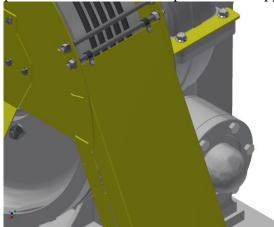
• Loosely (Whiz Bolts finger tight) attach the Bottom Extension Angles to the Lower Cover and slip the Lower Cover into place within the Upper Cover.
