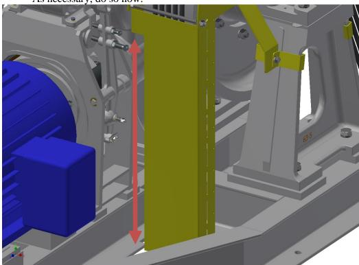
• Install the "P" Clamps to the lowest Retaining Rod above the Rope Gripper and attach the Cover (167 or 249) to the "P" Clamps with self-tapping screws. **Before continuing,** confirm the Cover was trimmed adequately and adjust as necessary.
