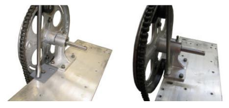
12. Unscrew stud for the motor mount tensioner.
