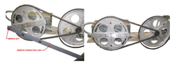
3. Remove 2 bolts on the door drive arm support assembly to separate door drive arm.
