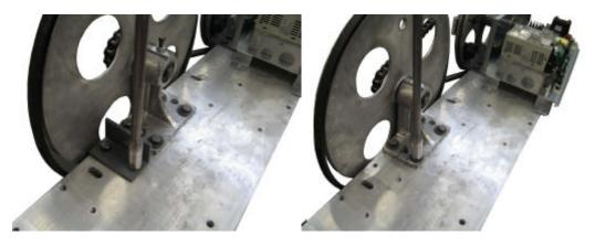
11. Slide operator controls enclosure out of the way. Remove 2 bolts securing the stop plate for drive pulley limit. Then remove 4 bolts securing the drive pulley assembly to the base.
