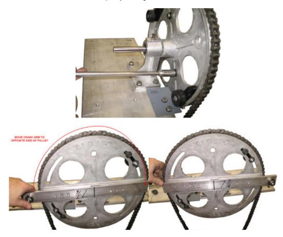
17. Reinstall stud for motor mount tensioner. (Ref. Step 13). Then follow reassembly in reverse order from steps 12-2.
