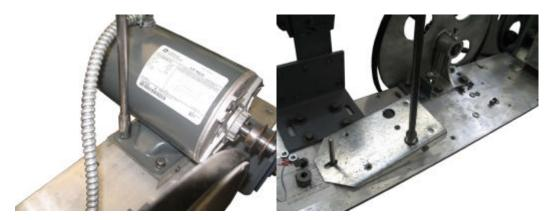
9. Remove 4 bolts holding drive arm support assembly to the base. <u>Note:</u> During reassembly in the opposite hand, you must remove the 3 bolts on the support assembly and shift to top half of the support over to the next set of holes. (if applicable)
