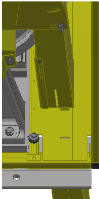
Figure 18: Machine Guard Rope Filler Panel Modification.
