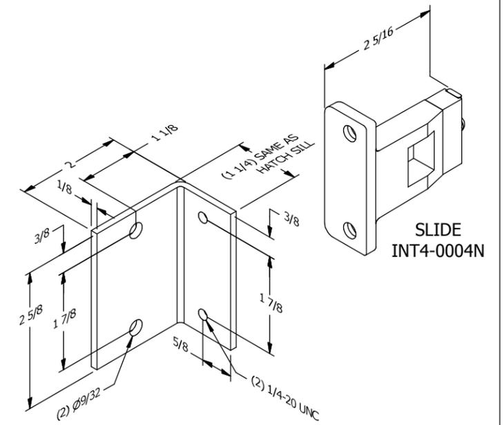
**"SN" LOCK AND CONTACT FLUSH MOUNTED DOOR & JAMB DRILLINGS & REINFORCEMENTS FOR SLIDING DOOR INSTALLATIONS**
