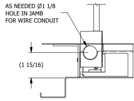
FIGURE 1 LOCK & CONTACT ARRANGEMENT
