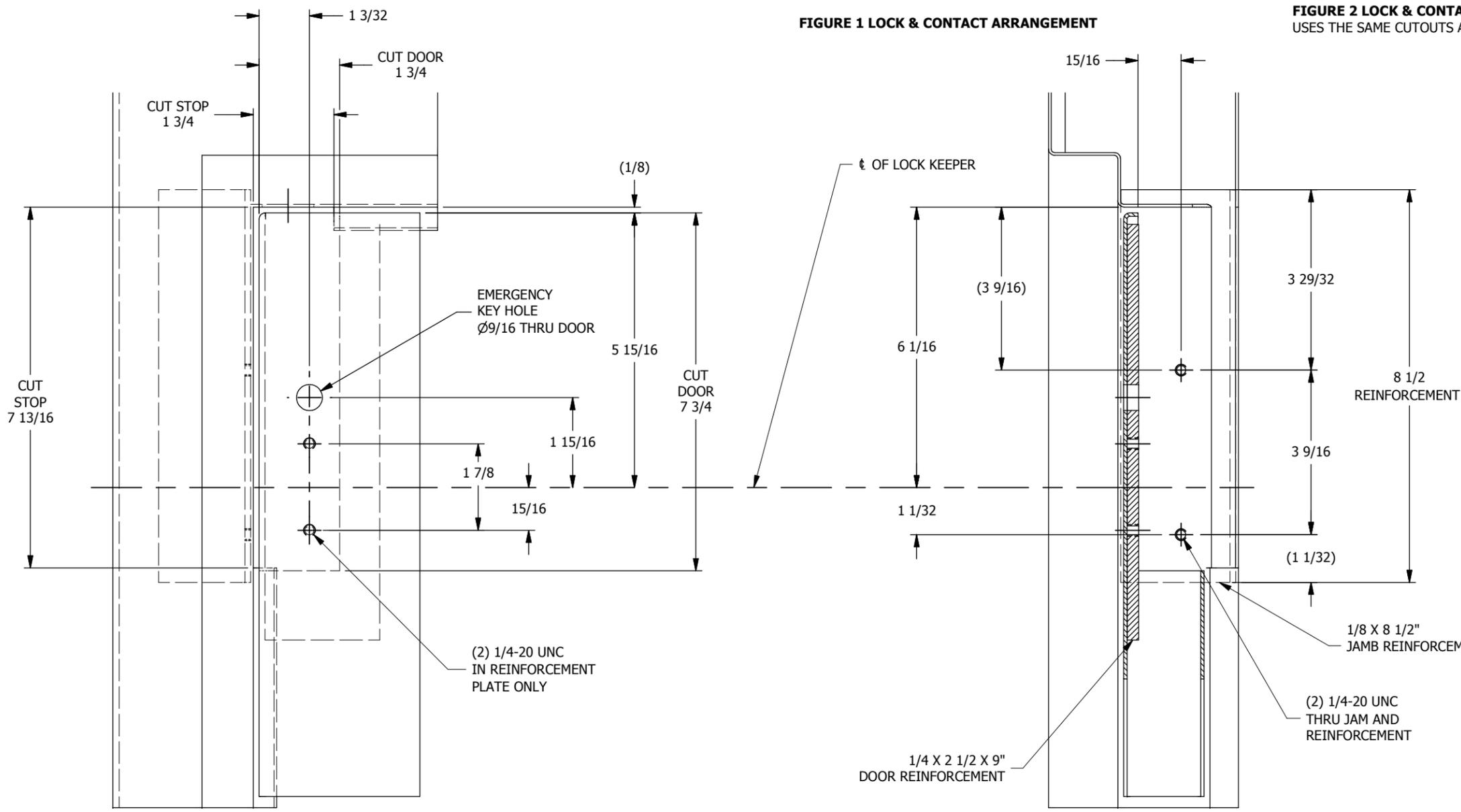
**"SN" LOCK AND CONTACT SURFACE MOUNTED DOOR & JAMB DRILLINGS & REINFORCEMENTS FOR SWINGING DOOR INSTALLATIONS**
